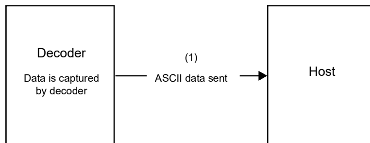
Figure 9-4 ACK/NAK Disabled and Unpacketed ASCII Data
