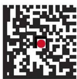
Figure 3-10 DS36X8-DP and DS36X8-DPA Aiming Pattern
