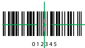
Figure 3-8 DS36X8-XR Aiming Pattern
